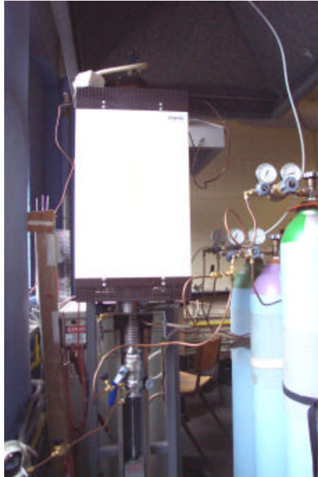
Figure 3.1: High temperature tube furnace for gas-slag-metal experiments.
