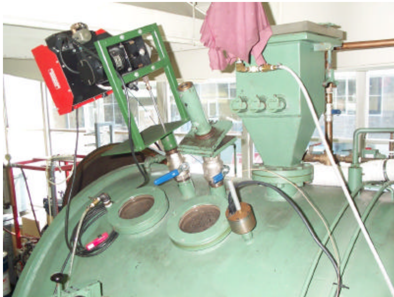
Figure 2.2: Induction furnace chamber ports. Top left clockwise: wire injection, hopper additions, pressure measurement/gas inlet, gas outlet (back right), 2 viewing ports, and pressure relief.
