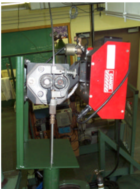
Figure 2.4b: Steel-clad calcium wire (5 mm diameter) seated in wire feeder.
