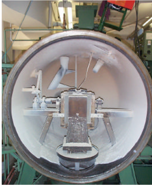
Figure 2.14: Induction furnace, after injection, showing extensive CaO fume coating.
