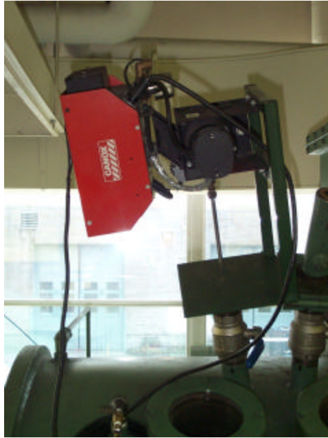
Figure 2.3: Wire feeding unit located on top of furnace chamber.
