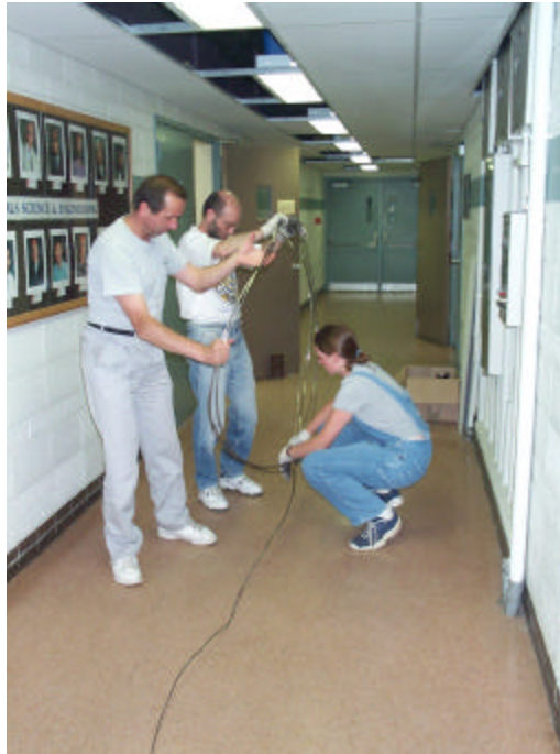
Figure 2.5: Uncoiling and straightening clad wire prior to injection experiments.
