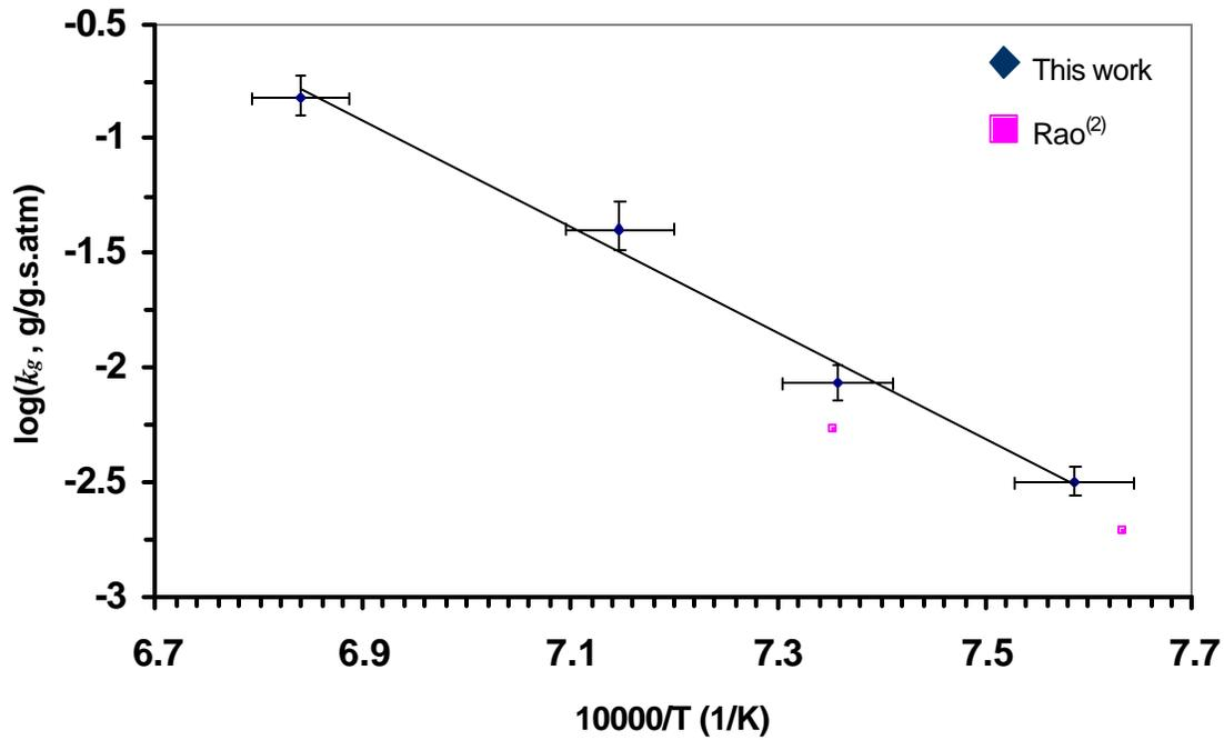
Figure 3: Intrinsic rate constants for oxidation of graphite in composite samples with wustite.
