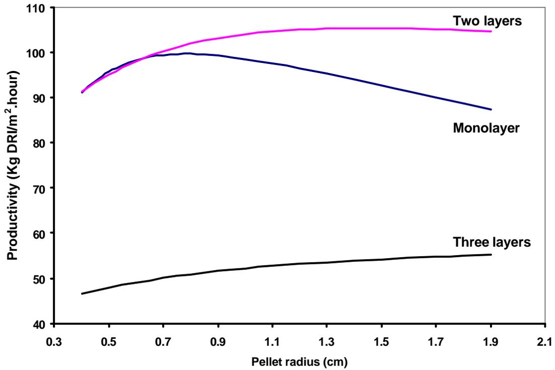
Figure 6: Predictions from the productivity model developed employing coal as reductant for typical RHF operational conditions. Reported productivities of RHF operations are usually between 70 and 90 Kg DRI/m<sup>2</sup>.hour at 90% metallization.
