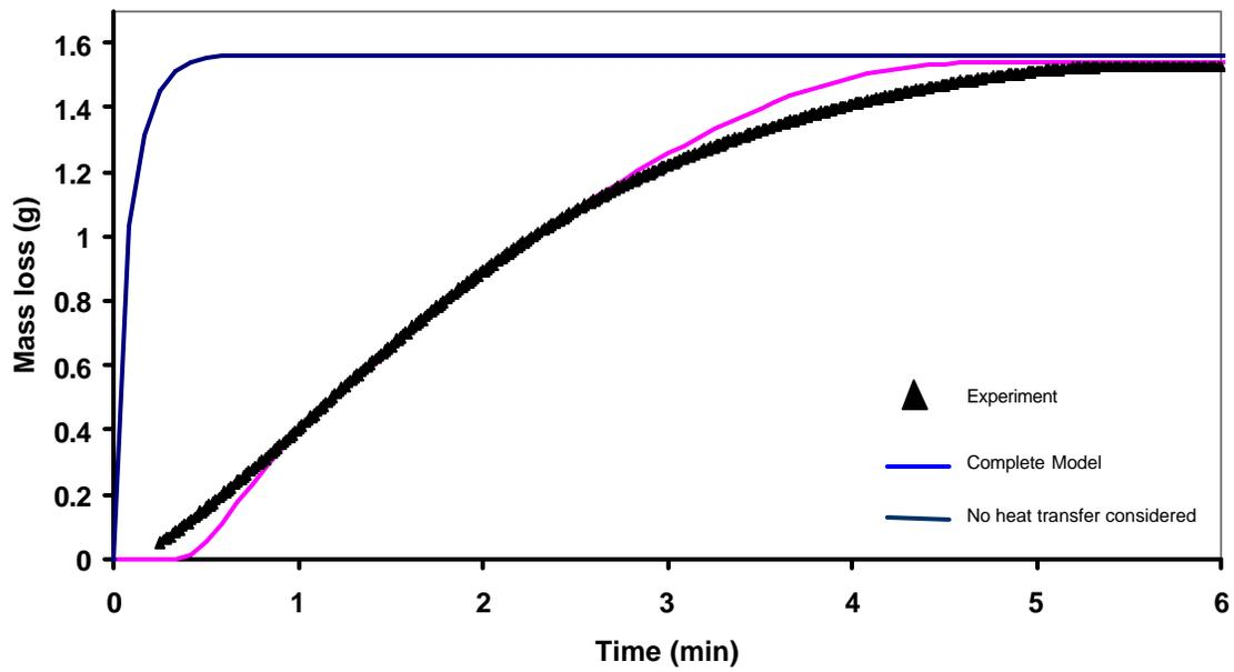
Figure 11: Comparison of experiment and pellet model for a pellet of wood charcoal and hematite. Isothermal model included for illustrative purposes. Large pellet with 3.86g reduced at 1280°C. Wood charcoal/hematite mass ratio of 0.1766.
