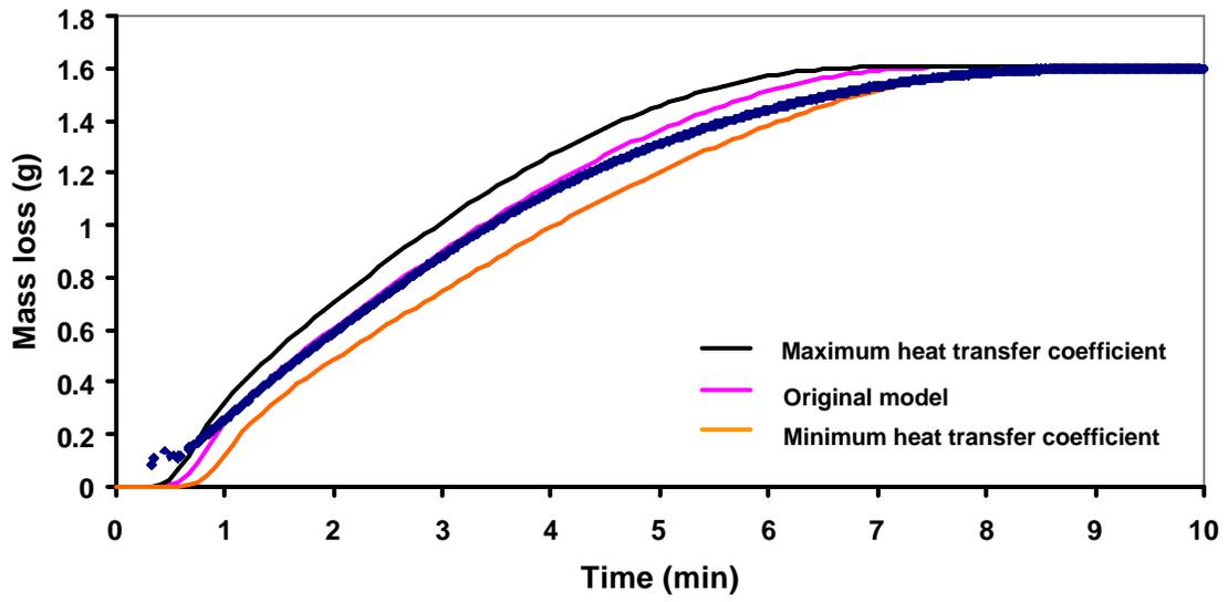
Figure 15: Effect of changes in external heat transfer coefficient on model predictions for a pellet of wood charcoal and hematite (4.04g at 1200°C).
