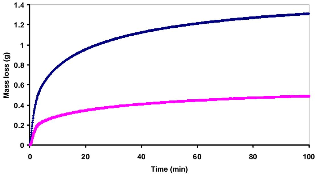
Figure 8: Typical measurements of mass loss with pellets of coal char and hematite at a mass ratio coal char/hematite of 0.177. (Pellets of 4.26 and 1.31g reduced at 1200°C).
