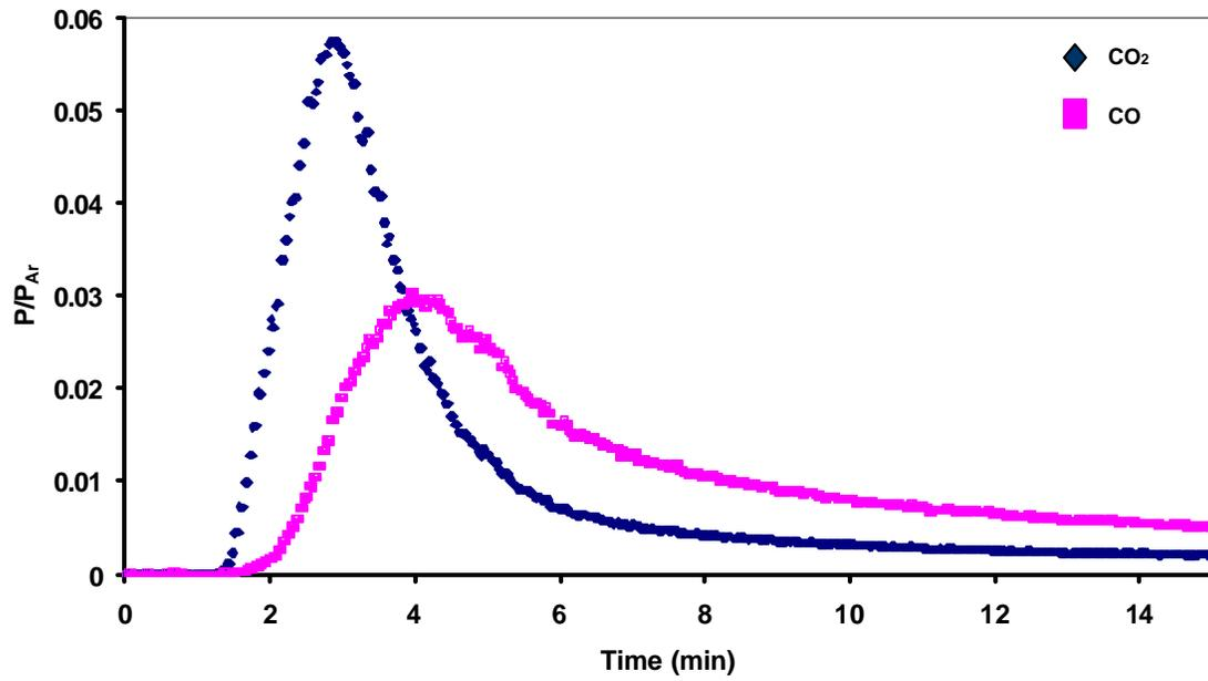
Figure 9: Off gas composition measurements from the experiment with large pellet of coal char and hematite. (4.26g at 1200°C).
