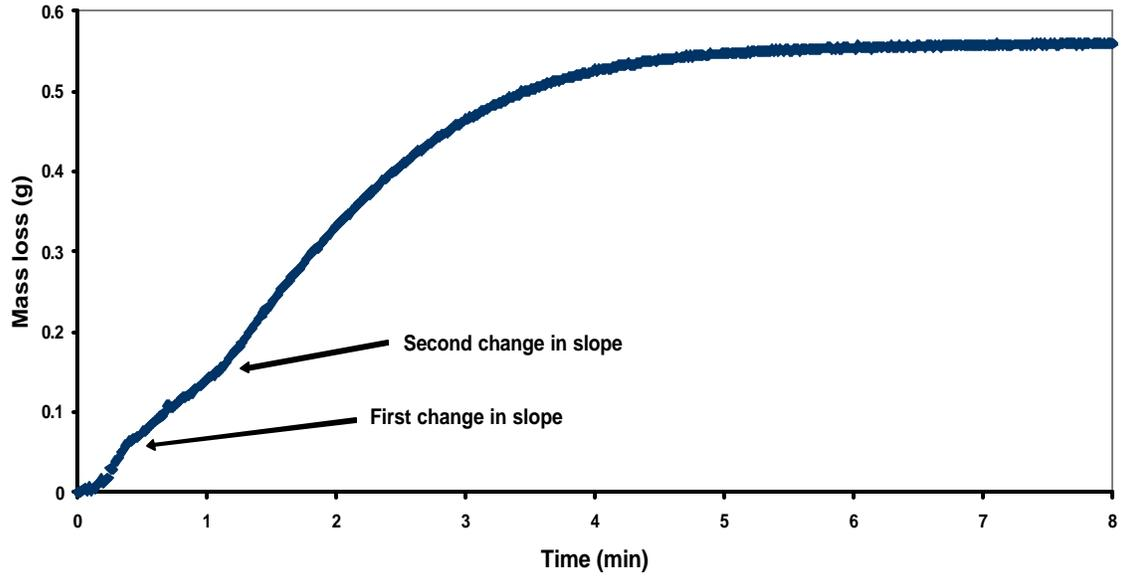
Figure 4: Typical measurements of mass loss with pellets of graphite and hematite showing two changes in reaction rate. (1.4g pellet at 1240°C).
