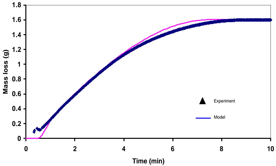
Figure 2: Example of validation of model developed for single pellets with laboratory measurements of reaction rates. Large pellet of 4.04g with wood charcoal and hematite reduced at 1200°C. Wood charcoal/hematite mass ratio of 0.1766.
