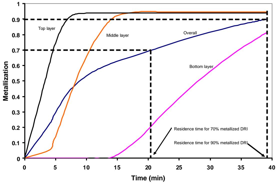
Figure 5: Example of determination of total residence time in RHF according to final metallization degree of charge considering three layers of pellets.
