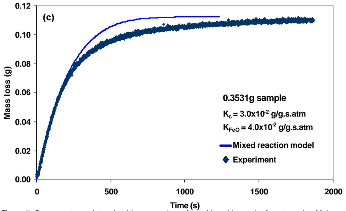
Figure 7: Rate constants determined in composites of graphite with wustite from taconite. Molar ratios of (a) 1/5, (b) 5/1 and (c) 1/1. Furnace at 1126°C.
