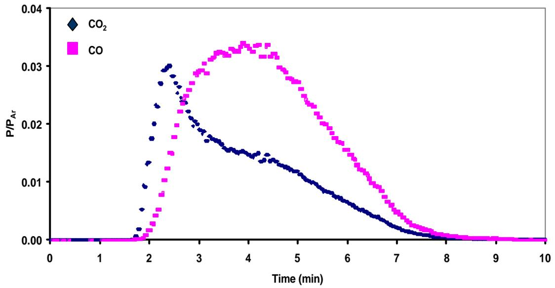
Figure 2: Off gas composition measurements from the experiment with large pellet of wood charcoal and hematite (4.04g at 1200°C).
