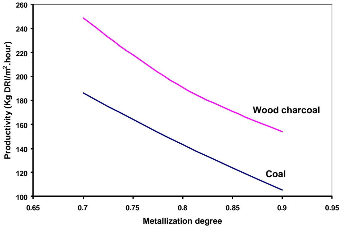
Figure 8: Estimated change in productivity of RHF operations according to metallization degree using coal or wood charcoal as reductant.
