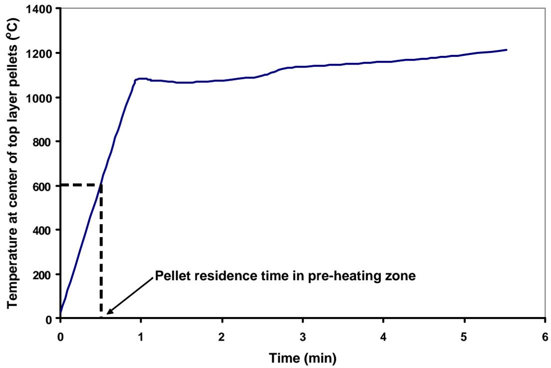
Figure 3: Example of determination of residence time in pre-heating zone considering a single layer of pellet with pre-heating temperature of 600°C.
