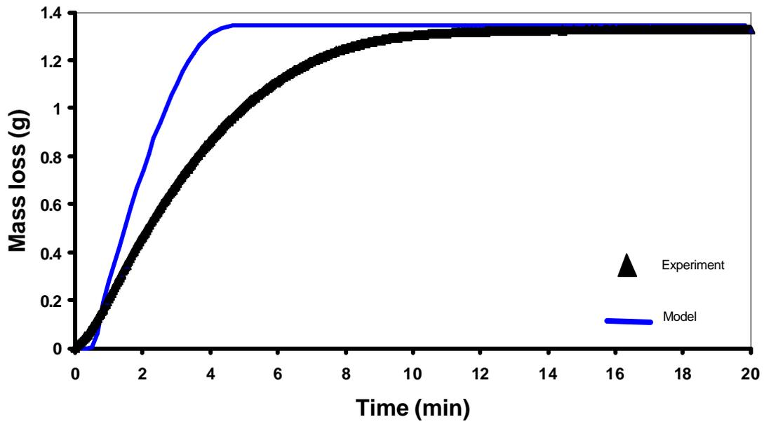
Figure 13: Comparison of experiment and pellet model for a pellet of wood charcoal and ore. Large pellet with 3.97g reduced at 1200°C. Wood charcoal/ore mass ratio of 0.1769.
