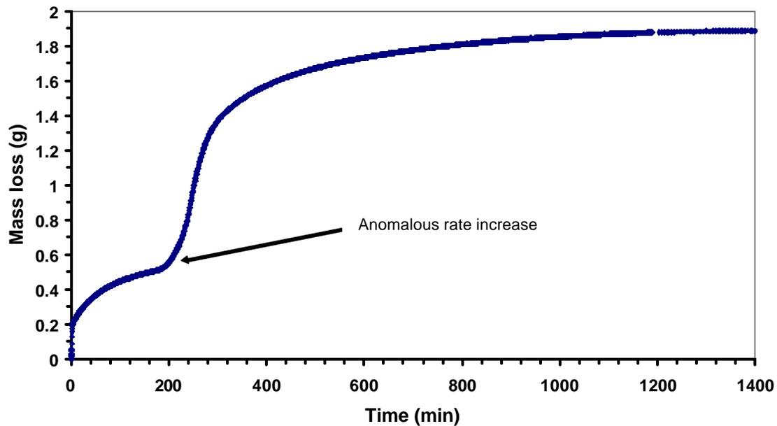
Figure 6: Mass loss measured during reduction of hematite with graphite showing anomalous rate increase. (5.28g at 900°C).
