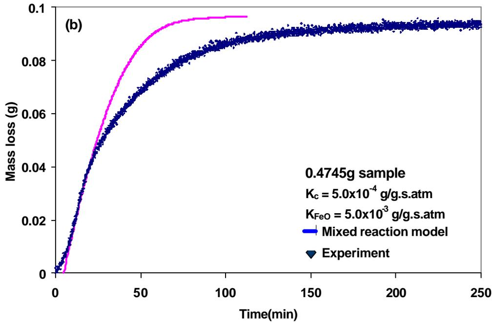
Figure 4: Iterative determination of rate constants by comparison of model results and measured mass losses at 940°C in samples with 1/5 carbon to wustite molar ratio (a) and 5/1 carbon to wustite molar ratio (b). Results for wood charcoal and taconite mixtures.
