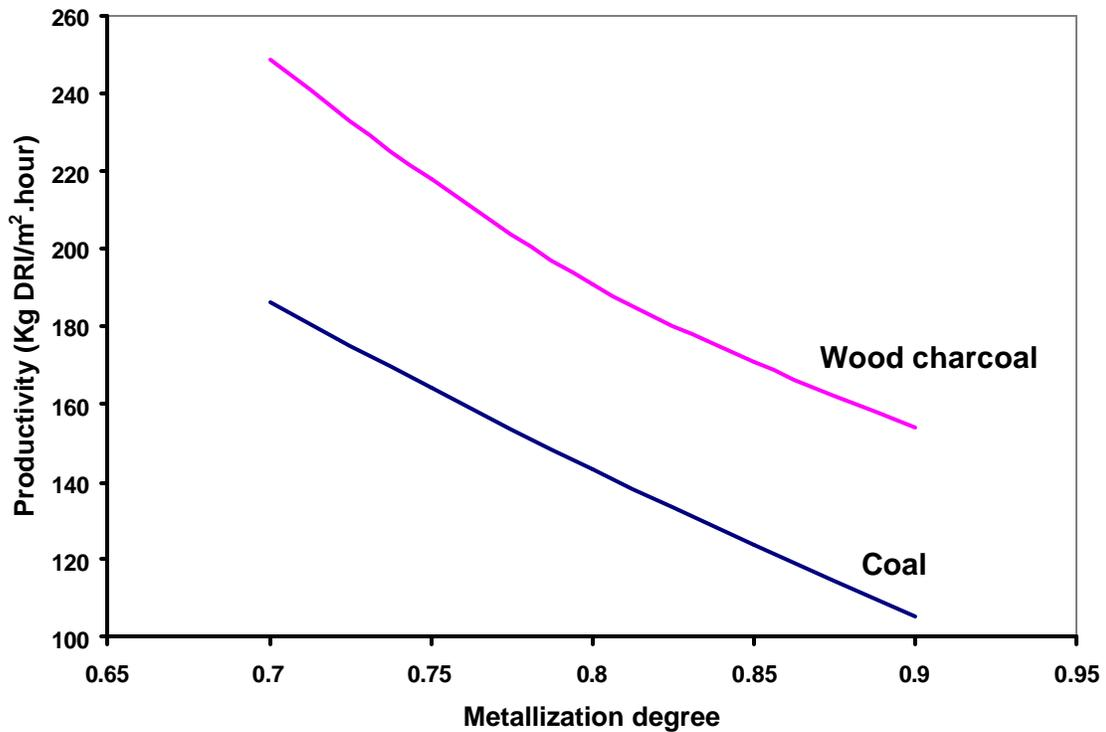
Figure 6: Estimated productivity of the RHF at different final degrees of metallization using wood charcoal and coal as reductant.
