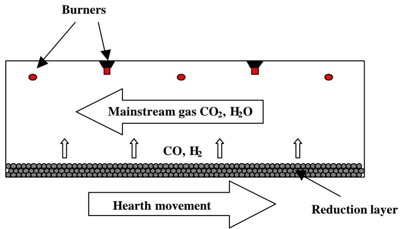
Figure 1: Rotary Hearth Furnace.
