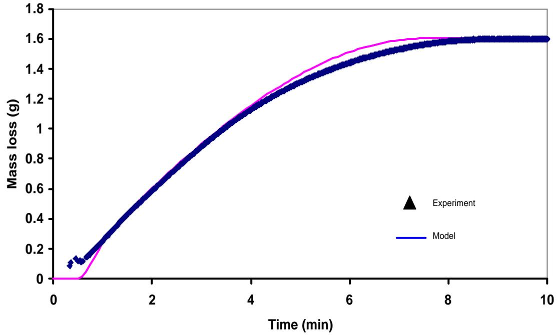
Figure 12: Comparison of experiment and pellet model for a pellet of wood charcoal and hematite. Large pellet with 4.04g reduced at 1200°C. Wood charcoal/hematite mass ratio of 0.1766.
