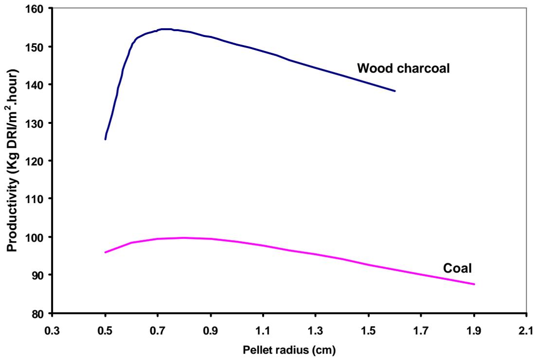
Figure 7: Results from simulations of operations using a monolayer of pellets containing coal or wood charcoal as reductant producing DRI 90% metallized.
