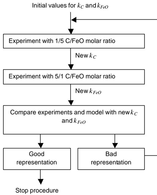
Figure 6: Schematic of procedure for determination of rate constants in mixed control reaction model.
