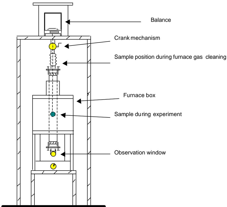
Figure 2: Experimental apparatus.
