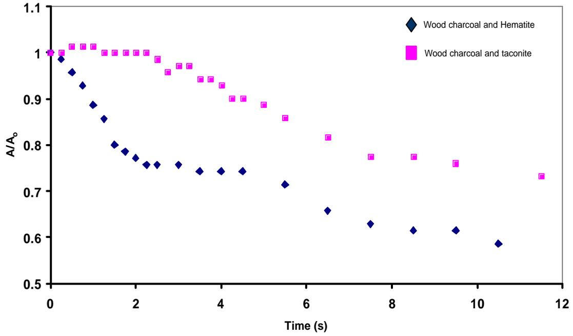
Figure 10: Measurements of cross section area of pellets of wood charcoal and hematite, and wood charcoal and North American Ore showing distinct shrinkage patterns.
