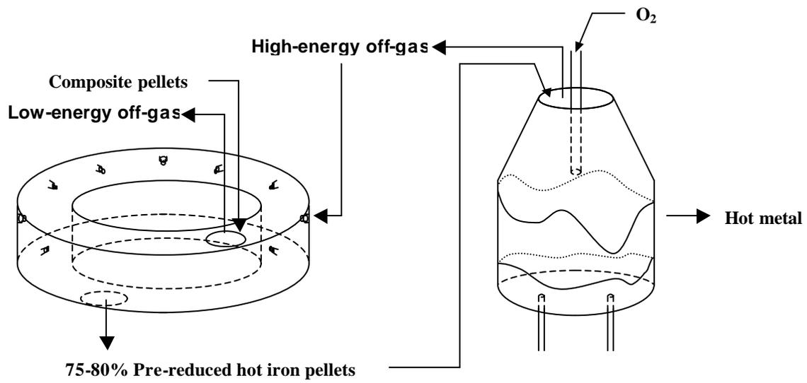
Figure 1: Schematic of the process proposed.
