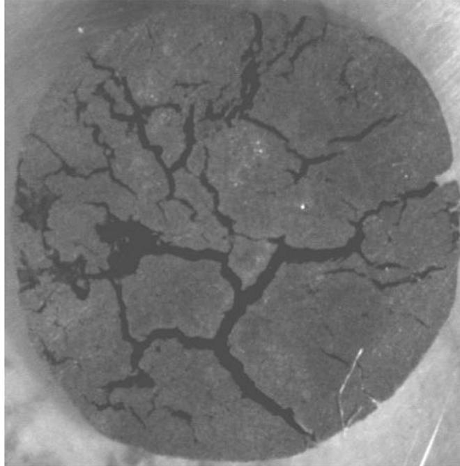
Figure 7: Fractured surface of a pellet of graphite and hematite reduced up to approximately 50% of mass loss showing no appreciable differences in reduction extent.
