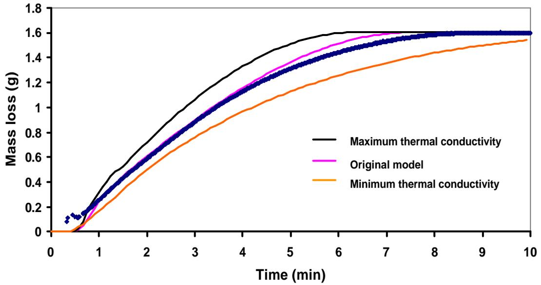
Figure 14: Effect of changes in effective thermal conductivity on model predictions for a pellet of wood charcoal and hematite (4.04g at 1200°C).
