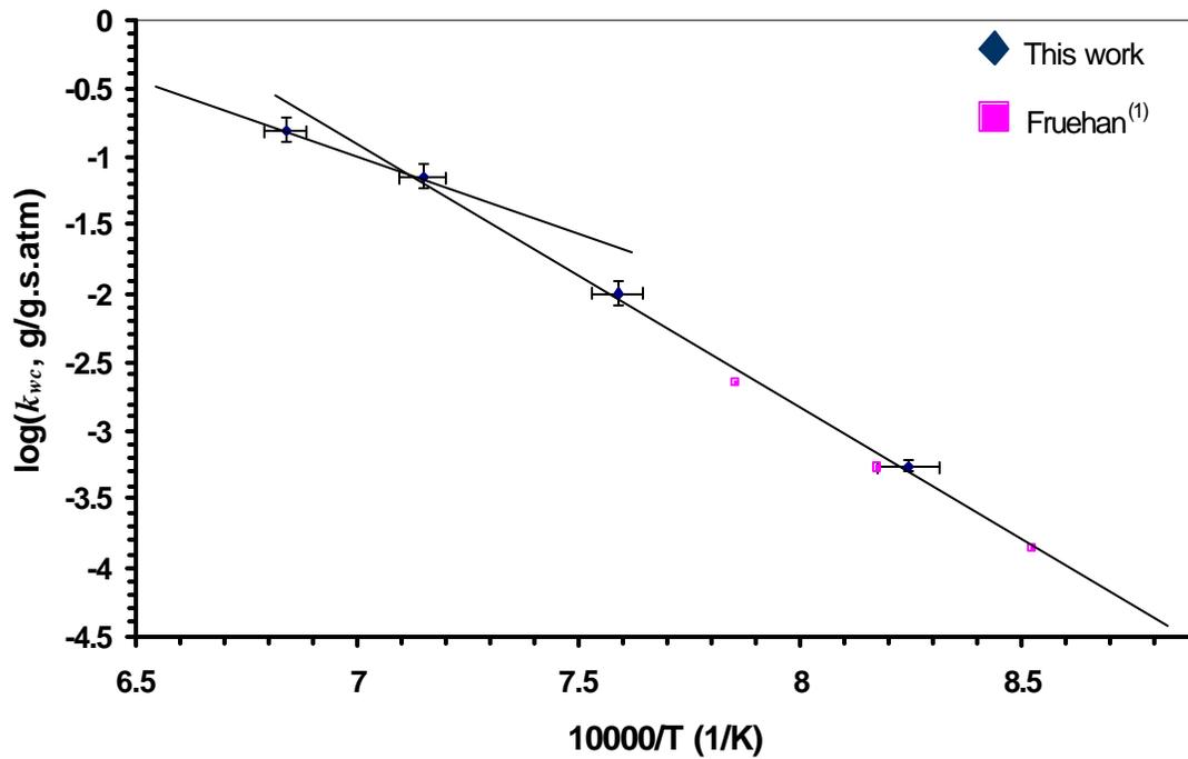
Figure 2: Intrinsic rate constants for oxidation of wood charcoal in composite samples with wustite.
