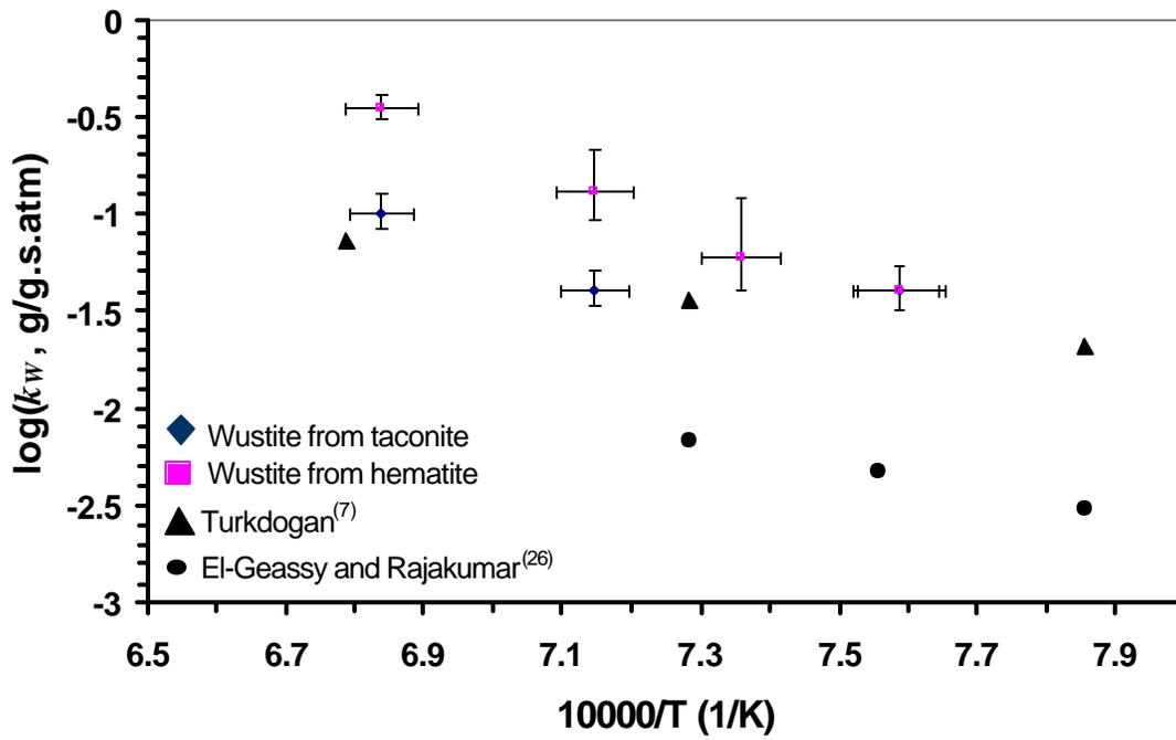
Figure 10: Comparison of intrinsic rate constants for reduction of wustite measured in this work with values from the literature.
