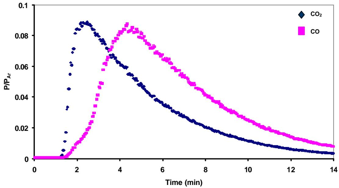
Figure 5: Off gas composition measurements from an experiment with a large pellet of graphite and hematite (3.98g at 1240°C).
