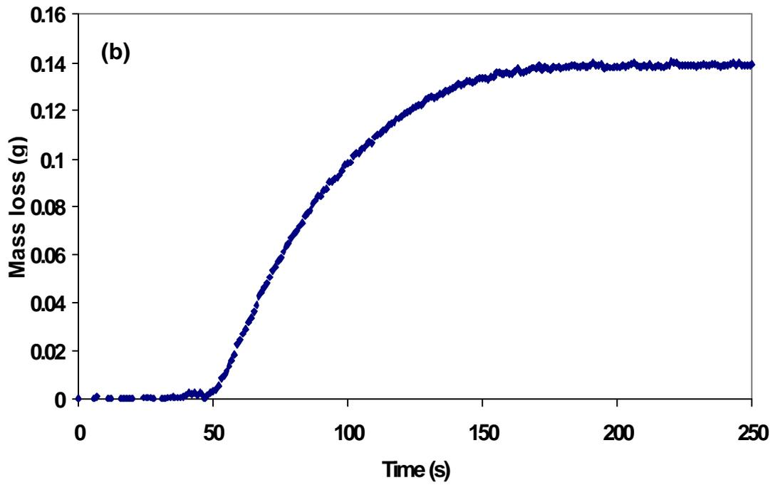
Figure 3: Typical results of measured mass change in samples with (a) wood charcoal and wustite from taconite and (b) graphite and wustite from hematite. 1126°C.
