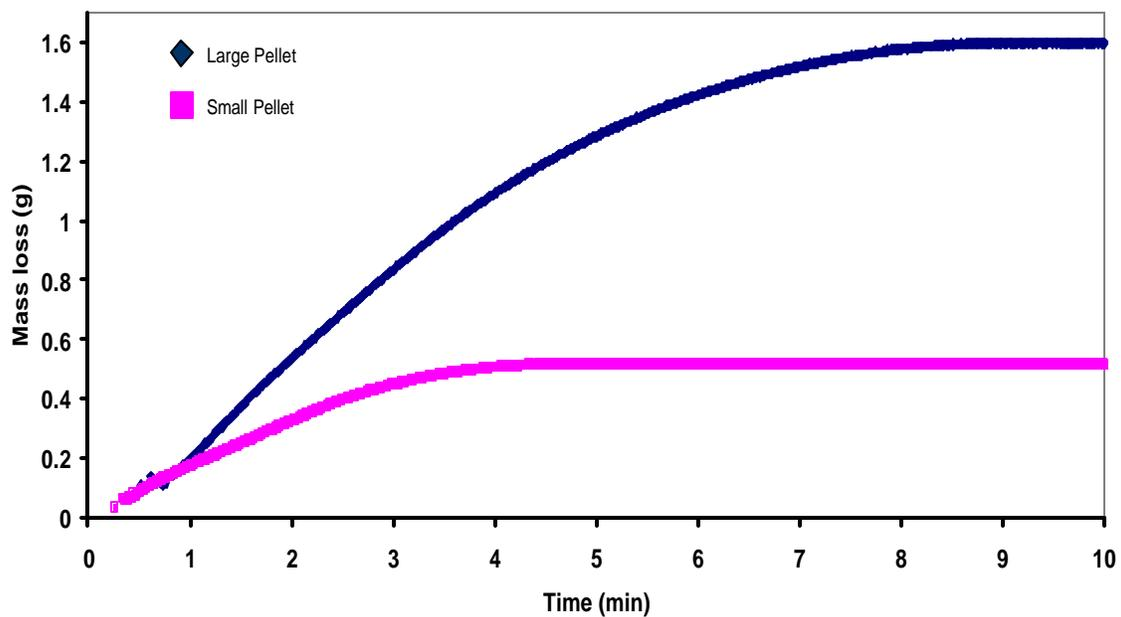
Figure 1: Typical measurements of mass loss with pellets of wood charcoal and hematite (4.04g at 1200°C).
