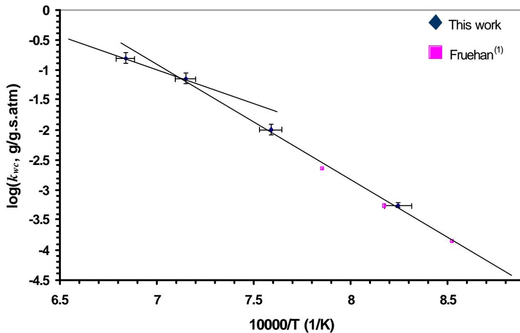
Figure 8: Temperature dependence of rate constants for oxidation of wood charcoal. Rate constants from Fruehan<sup>(1)</sup> relative to coconut charcoal.
