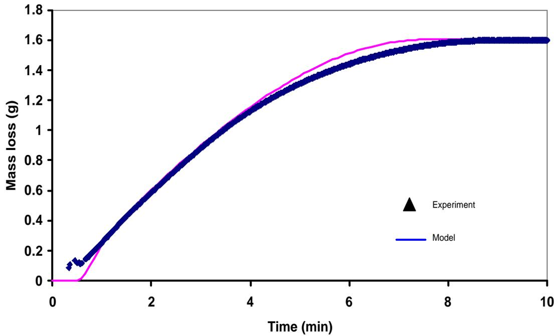
Figure 5: Comparison of experimental rates of reduction of composite pellets of wood charcoal and hematite and results from models with and without heat transfer.
