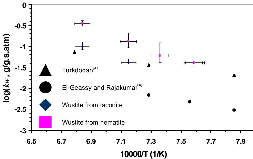
Figure 4: Intrinsic rate constants for reduction of wustite in composite samples with wood charcoal or graphite.
