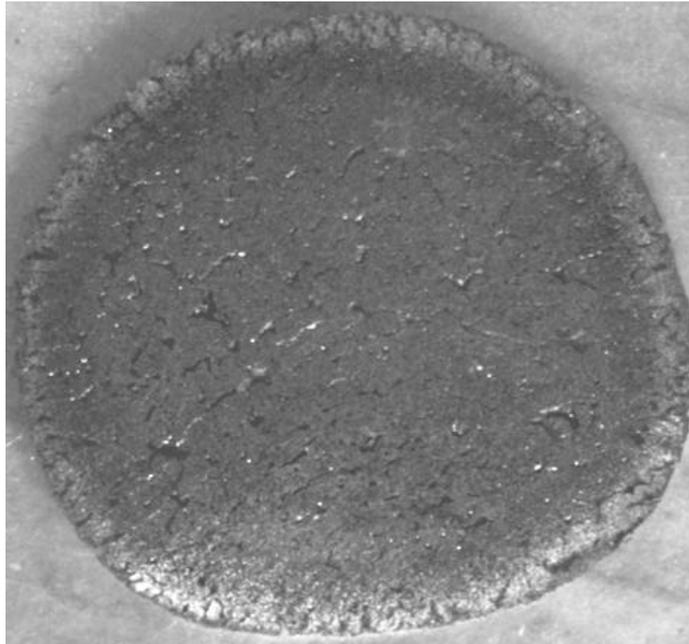
Figure 3 Fracture surface of pellet containing wood charcoal and hematite showing layer of reduced iron close to the surface.
