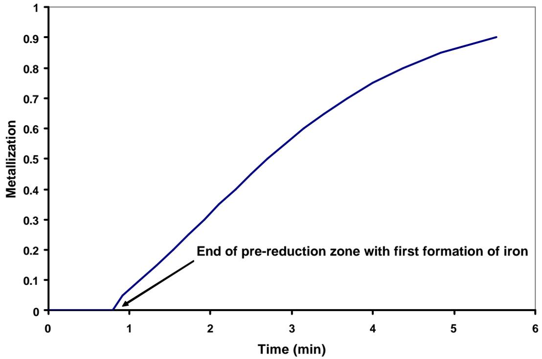
Figure 4: Determination of residence time in pre-reduction zone based on the limit of first formation of iron using a single layer of pellets containing wood charcoal and hematite.
