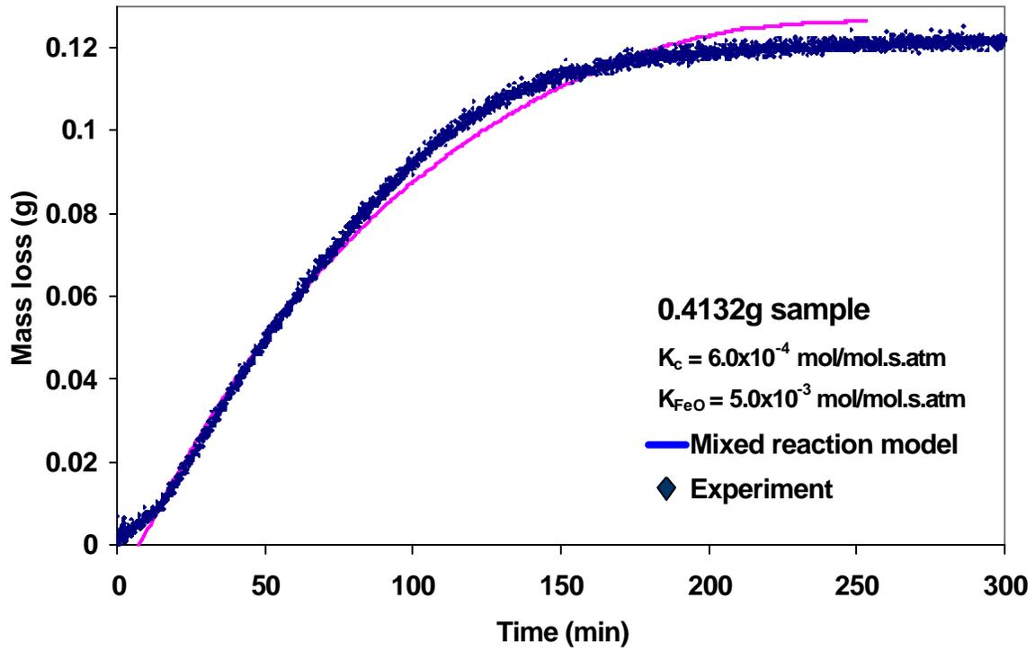
Figure 5: Validation of rate constants determined from experiments with low amounts of reactants using equimolar samples of carbon and wustite. Results at 940°C for wood charcoal and taconite concentrate.
