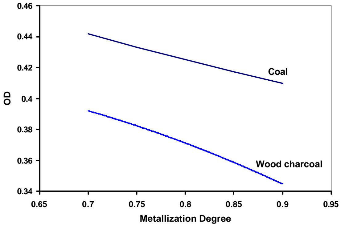
Figure 9: Comparison of estimated primary oxidation degree of gas in RHF for operations using coal and wood charcoal at optimum production rate.
