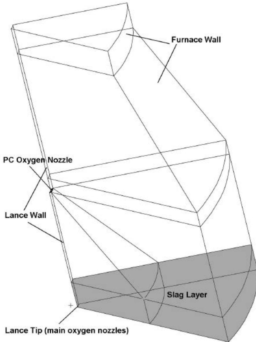
Figure 9. Block structure of the BOF post-combustion model
