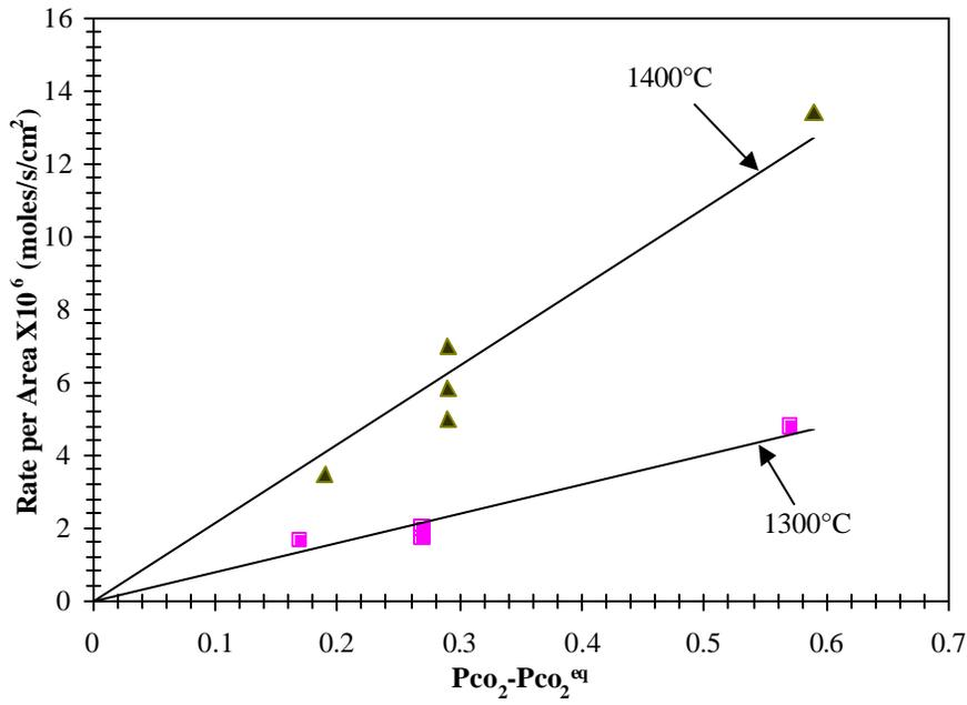
Figure 1: The linear oxidation rate plotted versus the partial pressure of CO<sub>2</sub> for 1300°C and 1400°C,  $P_{CO_2} + P_{CO} = 1$
