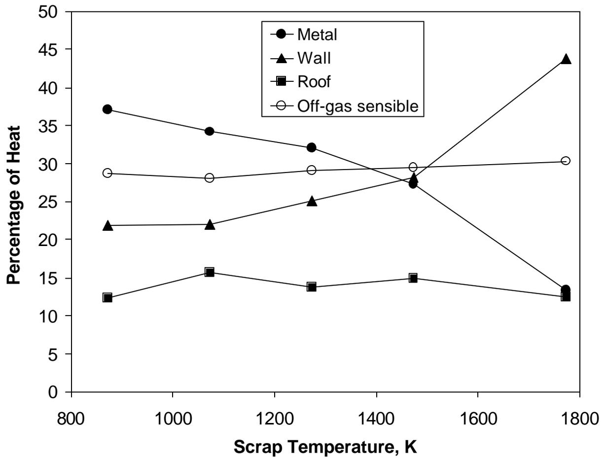
Figure 7. Variation of heat distribution with scrap temperature.
