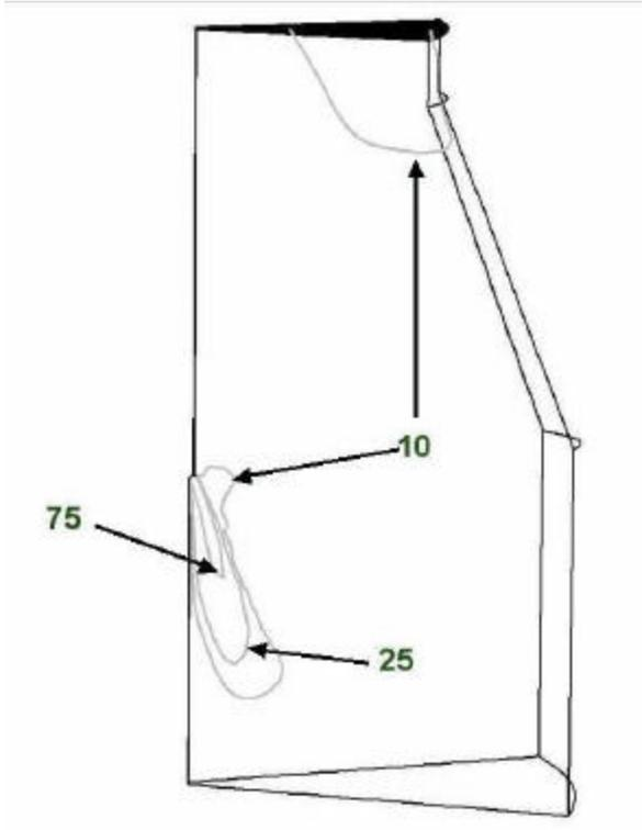
Figure 13. Velocity profile (m/s) for post combustion (Base Case)
