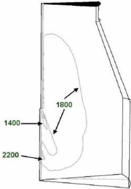
Figure 12. Temperature, ( $^{\circ}\text{K}$ ) for post combustion (Base Case)
