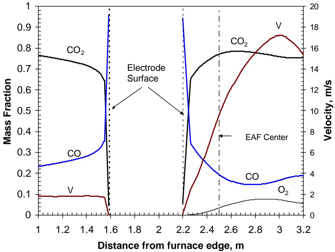
Figure 6. Profile of CO, CO<sub>2</sub>, O<sub>2</sub>, and velocity along a line, which is 1.5 m above the liquid metal level and crossing the centers of the northwest electrode and the furnace.
