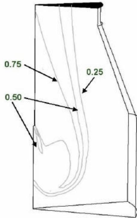
Figure 11. CO<sub>2</sub> fraction for post combustion (Base Case)
