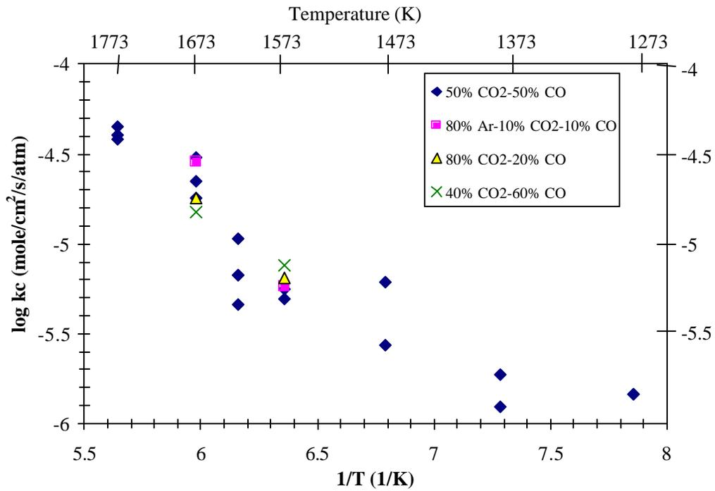
Figure 2: Kinetic rate constants for CO<sub>2</sub> oxidation from current research
