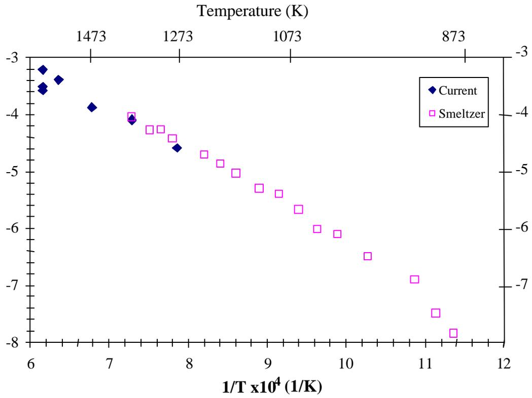
Figure 3: Parabolic rate constants from the present work and from Smeltzer
