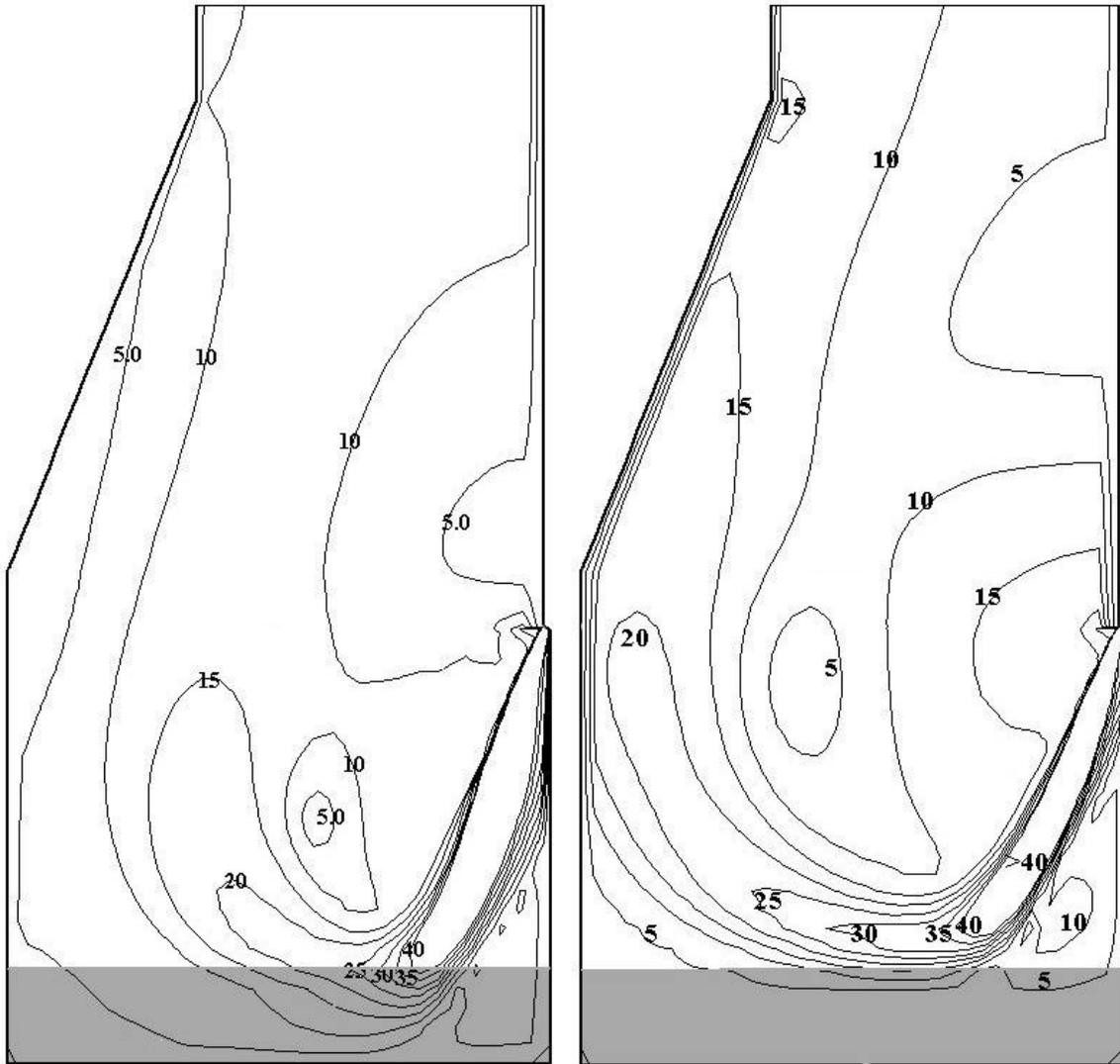
Figure 10. Velocity profile on the vertical plane crossing the PC nozzle center with slag resistance of (a) 10 and (b) 1000  $kg/m^3s$
