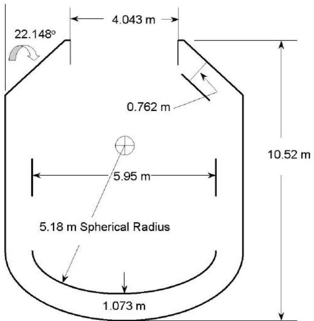
Figure 8. Schematic of the BOF Furnace
