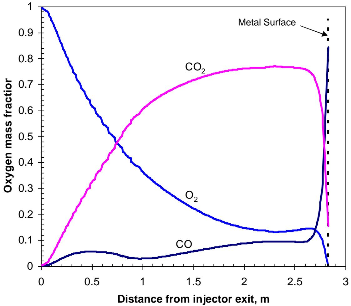
Figure 5. Oxygen, carbon monoxide and carbon dioxide profiles at the center of the west jet.
